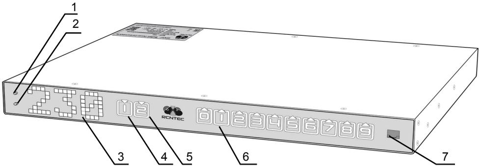
Fig. 4. Elements on the front panel of RPCM 1502 (16A) and RPCM 1532 (32A)
